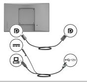
Connected to an HP Retail System or PC without a 12 V powered USB port.
